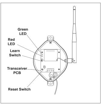
Figure 20. PDA Transceiver J-Box - Internal View
